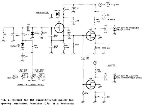
MV1652 or equivalent. Typical tuned circuit values for three popular vfo ranges are listed in table 1. Transistor selection is discussed in the text. R2 is a Beckman model 7426 RIK Helipot; R1 and R3 are Beckman Helitrims, model 78LRIK or equivalent.
